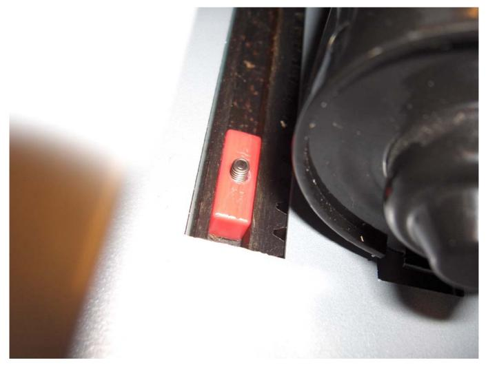
Assemble all parts backwards of the way the disassembly was done and test if the height limit is set correct. If not, disassemble and adjust again.
