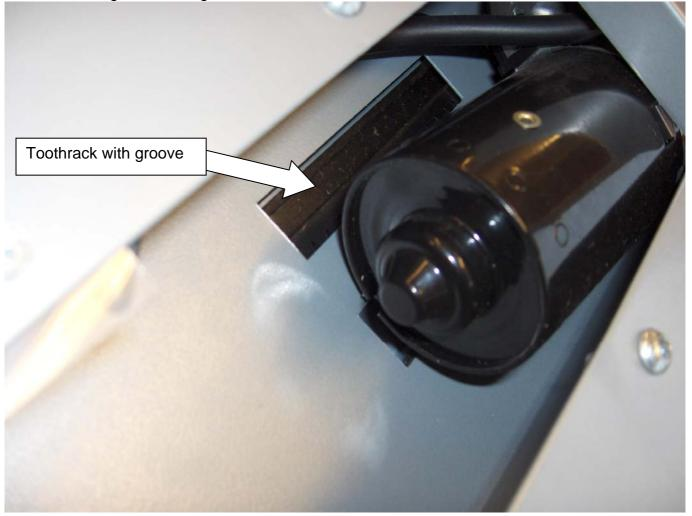
Install the red height limiter into the toothrack groove at the wanted height and tighten the screw:
